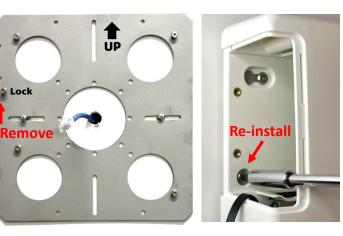
Install optional wire cage and both locking plates using a T10 Torx security bit.
