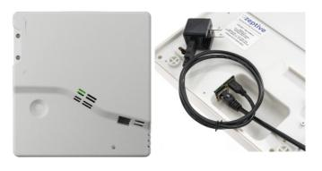
Remove locking screw and battery door. Slide device onto baseplate mounts and re-install locking screw.
