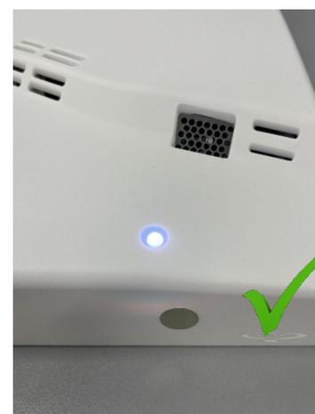
**NOTE:** This will put the device in reconfigure mode for ~5 minutes and the LED color will alternate between Blue and White. The process can be repeated with the magnet if it doesn't connect in time.
